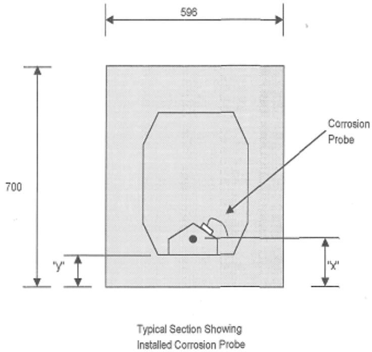
Figure VII Location of LPR probes in beam soffits
