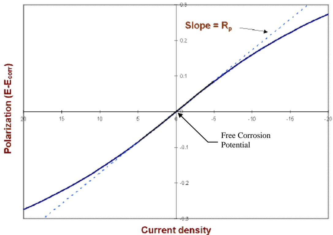
Figure I Polarisation in relation to current density
