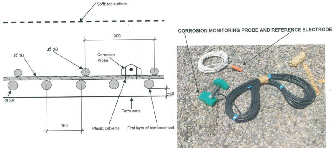
Figure XI Design details for probe locations
